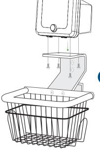
Align holes on bottom of the ADView 2 with the four holes on the mounting bracket as shown.
