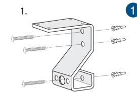
Attach wall bracket to wall before assembling basket. For optimum viewing, it is suggested that you measure 60" from the floor to the top of the wall mounting bracket (or adjust as needed). Once positioned to desired height, mark screw positions on the wall making sure bracket is level. Screw in the three supplied screws (5600-HW-01) firmly into a stud, or use the three supplied mollies and secure to the wall.
