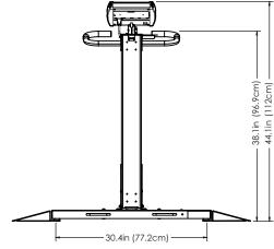
**6550 Capacity** 1,000 lb x 0.2 lb / 450 kg x 0.1 kg **6550KGEU Capacity** 300 kg x 0.1 kg (OIML EC Class III)
