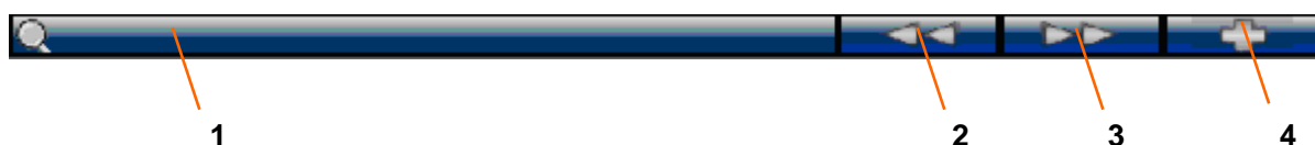
Figure 8-2 Trace control tools
