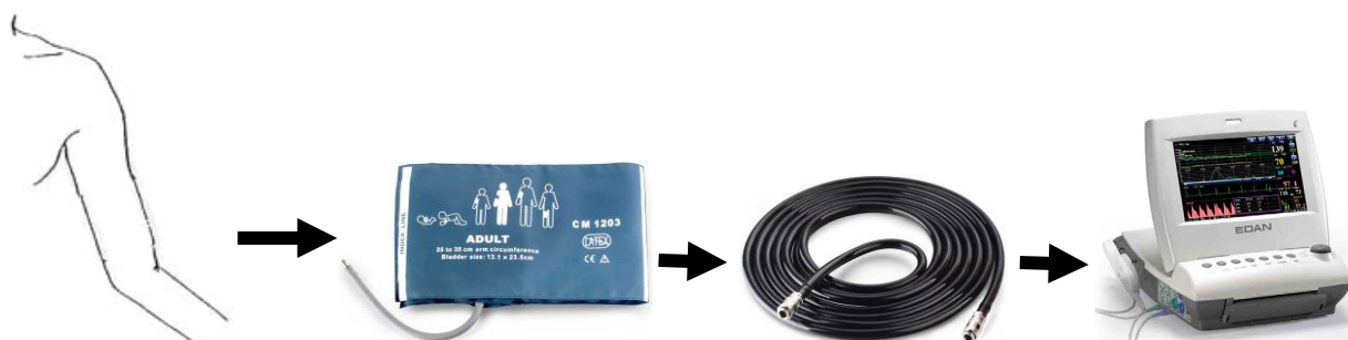
Figure 9-5 Connection for NIBP Measurement
