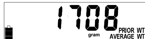
Figure 9: Motion detected during weighing
