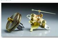
requirements under ANSI SP10. Machined from copper berrilyum, gears and diaphragms are pre-aged to ensure stability, even under the toughest environments. Accuracy of EACH gauge is tested not once, not twice but three times; then tested again in our own facility prior to final assembly.
