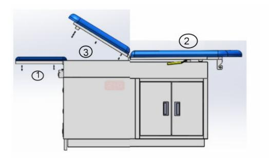
Push the pullout shelf with uphostery at the bottom of the knee board frame, and then put the knee board section flat as below picture.
