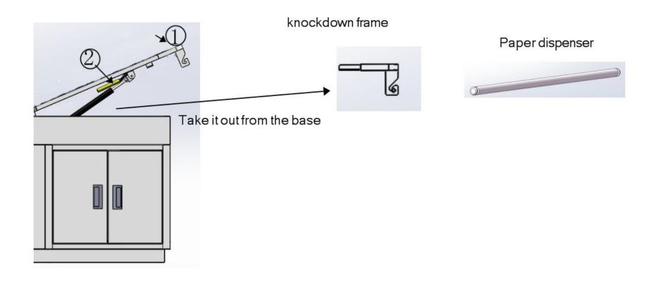
Insert the knockdown frame slide in the tube of backrest frame.
