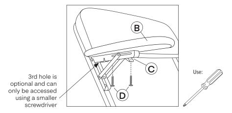
To ensure you have the correct Arm Pad (B), the inner point of the Arm Pad (B) should measure 0.12" (3 mm) from the bracket, and the outer point of Arm Pad (B) should measure 0.2" (5 mm) from the bracket.
