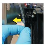
**9** Push down and pull the rinsing head to remove it from the rocker.
