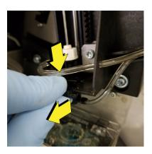
${\bf 10}\,$  Pull up the probe to remove it from the rinsing head.
