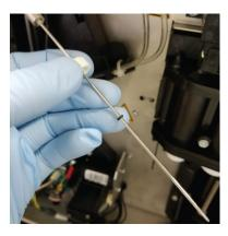
**6** Install this assembly on the rinsing head and screw back the black probe guide.
