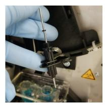
**NOTE** The white spacer may or may not be seen with the removal of the aspiration probe. Be careful not to lose the spacer if it is removed.
