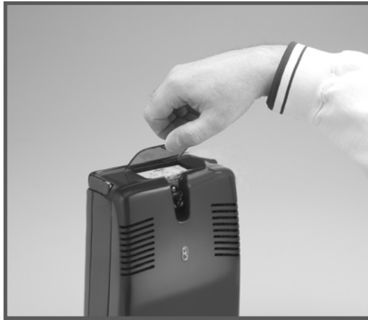
Figure 16: Lifting Dust Cover on Keypad Display
