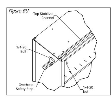
Step 63: Remove (1) 1/4-20 x 3/4" hex bolt and nut from far left and far right of each top stabilizer channel. Insert overhead safety stop into stabilizer channel and secure using the same 1/4-20 hardware as shown in Figure BU.
