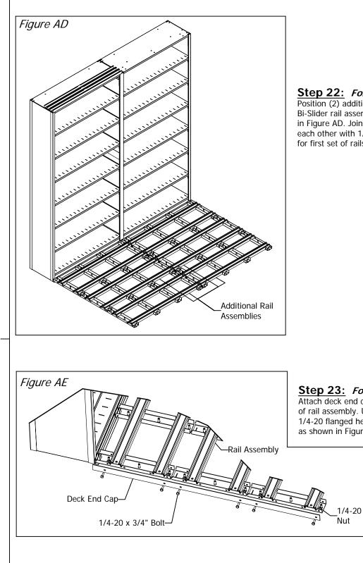
Step 22: For QuadSlider Systems Only Position (2) additional rows of rail assemblies in front of
