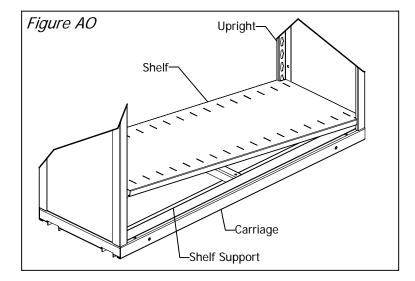
Step 30: Install bottom shelf by tilting as shown in Figure AO. It should then lie flat on shelf supports and reinforcement(s).
