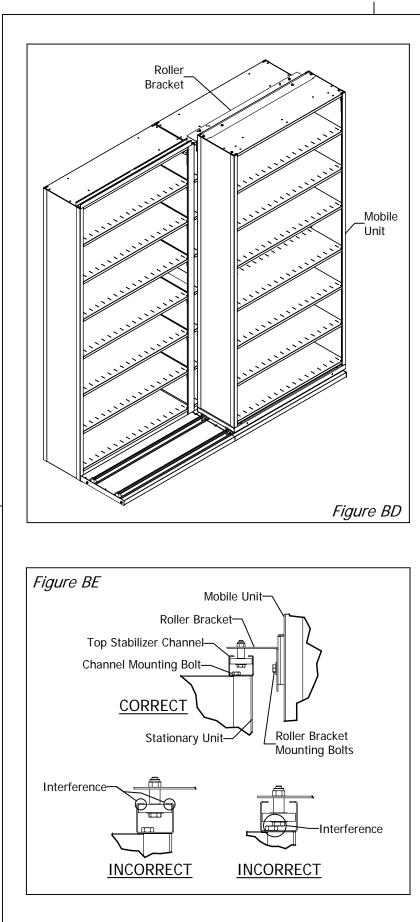
Step 45: Place assembled mobile unit on tracks of rail assembly in front of stationary unit that does not have a top stabilizer channel installed (See Figure BD).
