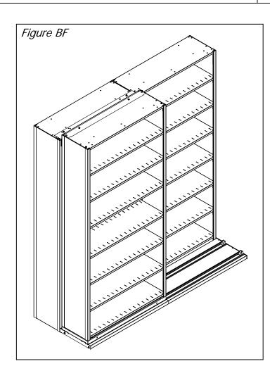
Step 47: Move mobile unit so that the roller bracket is completely engaged within the row of installed top stabilizer channels on the stationary units as shown in Figure BF.
