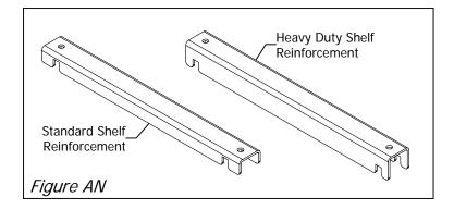
**Step 29:** Install heavy duty shelf reinforcements for the bottom shelf as shown in Figure AM. See Table 2 for proper number of reinforcements. Figure AN shows the visual difference of a standard shelf reinforcement compared to a heavy duty reinforcement.
