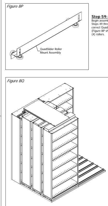
Begin assembly of a new QuadSlider mobile unit by following Steps 49 through 55. For Steps 53, 54, & 55, be sure to use the correct QuadSlider components in place of TriSlider components (Figure BP shows correct QuadSlider roller mount assembly with
