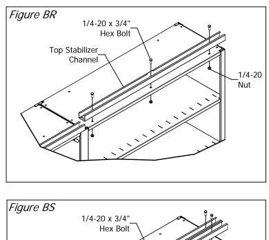
Step 62: Attach remainder of top stabilizer channels to stationary units with 1/4-20 x 3/4" hex bolts and 1/4-20 flanged hex nuts. Refer to Figure BR for BiSlider systems; Figure BS for TriSlider systems; and Figure BT for QuadSlider systems.
