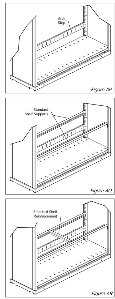
**Step 31:** Install back stop for bottom shelf. Count up three complete keyholes from top of shelf and place rivets of back stop into these keyholes (See Figure AP).
