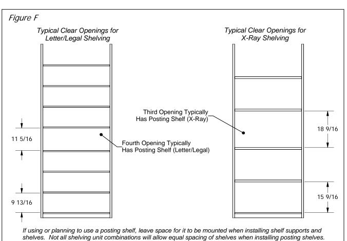
shelves. Not all shelving unit combinations will allow equal spacing of shelves when installing posting shelves. One opening will need to be larger than the rest. Check with your dealer or supplier for the correct choices of uprights and shelf openings required when a posting shelf is desired.
