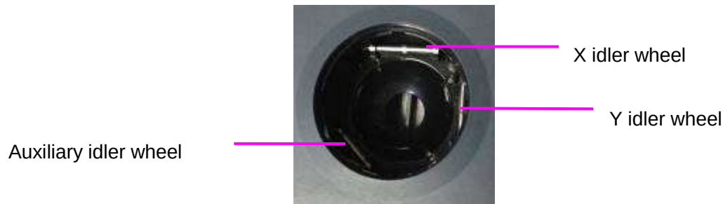
Figure 13-2 X, Y and the Auxiliary Idler Wheels
