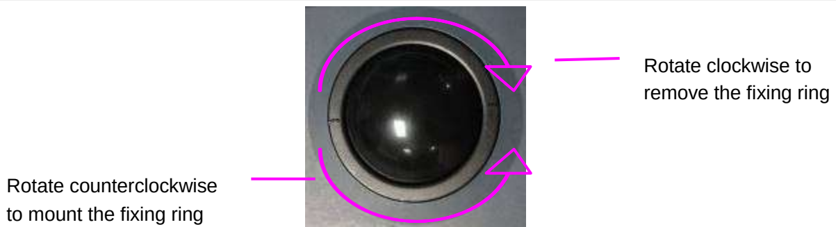
Figure 13-1 Assembling and Disassembling Trackball
