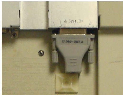
Figure A2-4 A Protocol Converter Used on a Monitor
