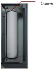
5) Pull the paper out with the grid side facing the thermal print head, and replace the casing on the recorder.
