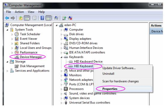
d) Click on the **Details** tab in the HID Keyboard Device Properties window. View the vector ID (VID) and the product ID (PID). Take the following figure for example, the vector ID is 04B4, and the product ID is 0100.
