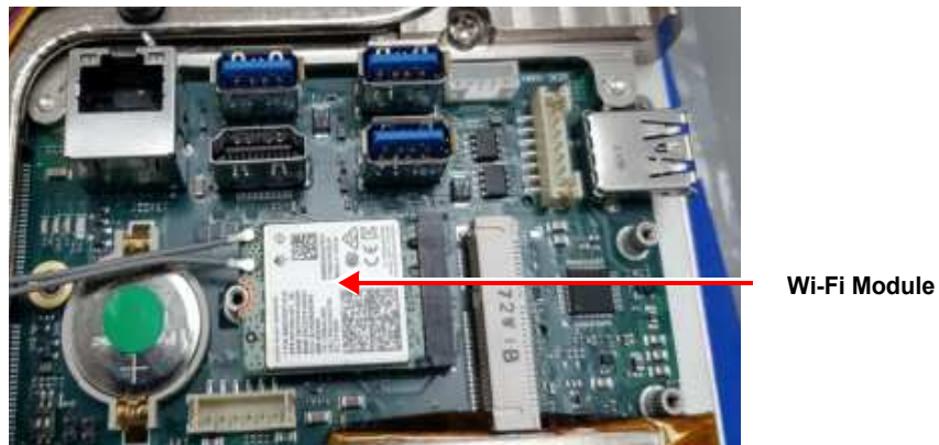
Figure 8-96 Wi-Fi Antenna Cables
