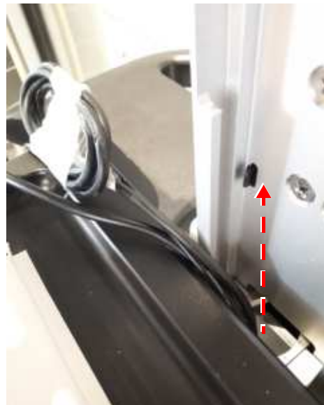
Figure 8-142 Pull ECG USB cable upwards through the pole
