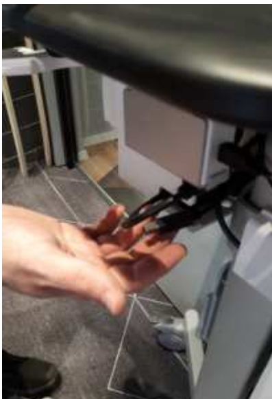
Figure 8-139 Pull Printer USB cable upwards through the pole
