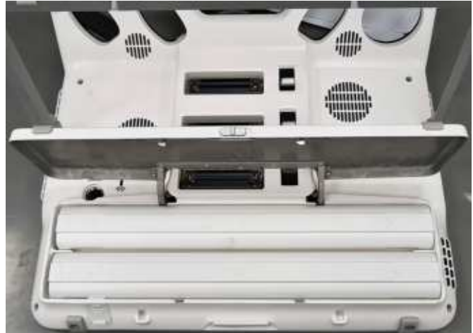
Figure 8-72 Opening Battery Compartment Cover
