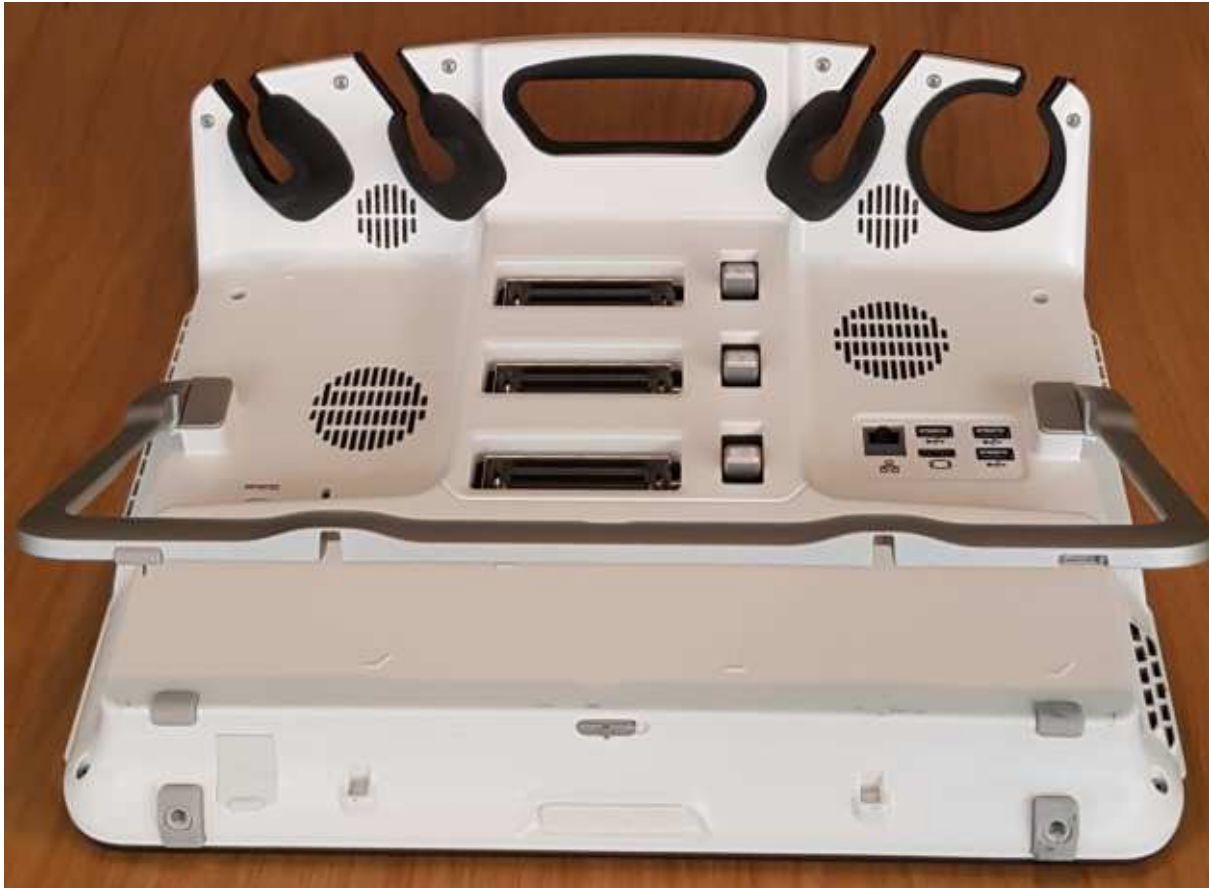
Figure 4-62 Open System's Back-Cover Support
