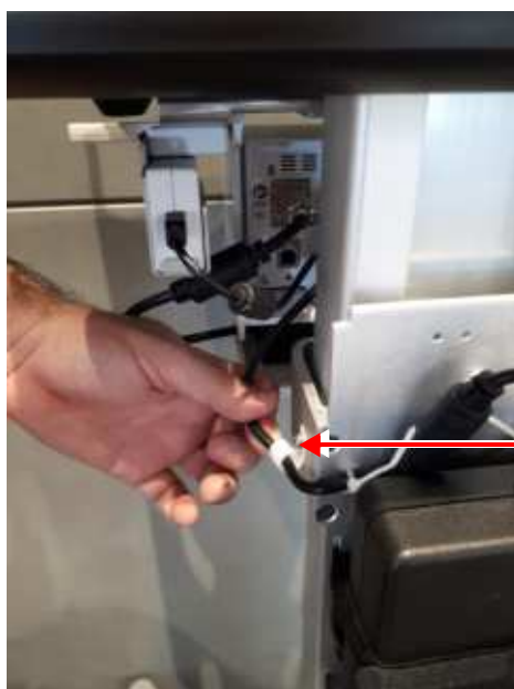
Figure 8-145 Release power cable from P clip
