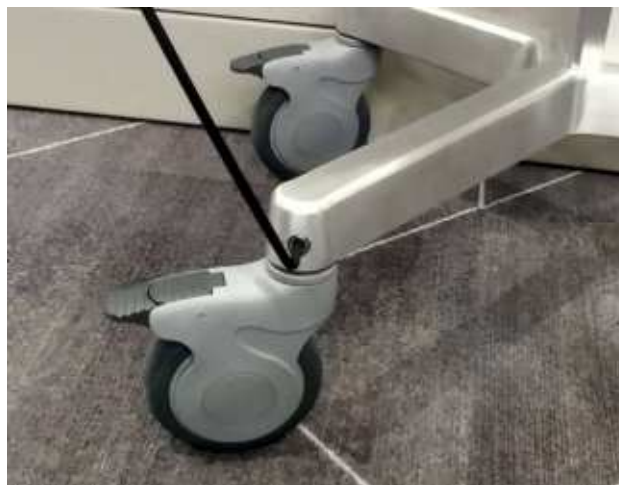
Figure 8-125 Removing Cater Cap and Holding Screw
