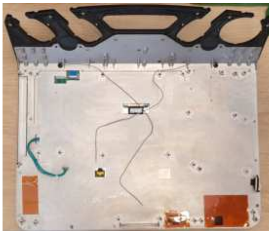
Figure 8-108 Front Display Assembly Removed
