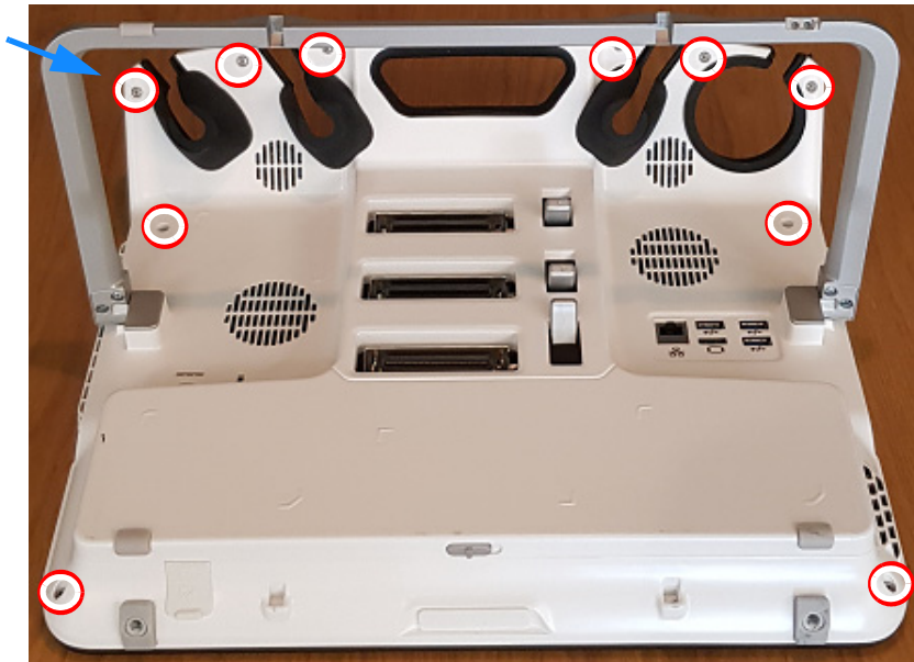
Figure 8-74 Releasing 10 captive Screws
