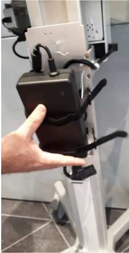
Figure 8-146 Remove Power Supply
