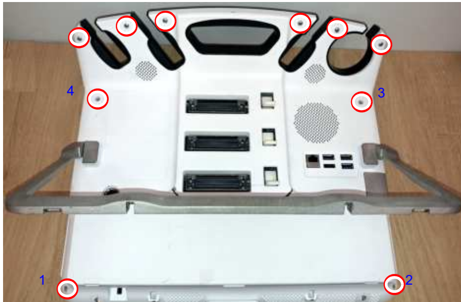
Figure 8-76 Fastening 10 captive Screws: Order
