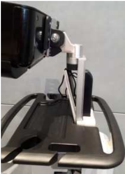
Figure 8-141 Remove Cable Plastic Cover
