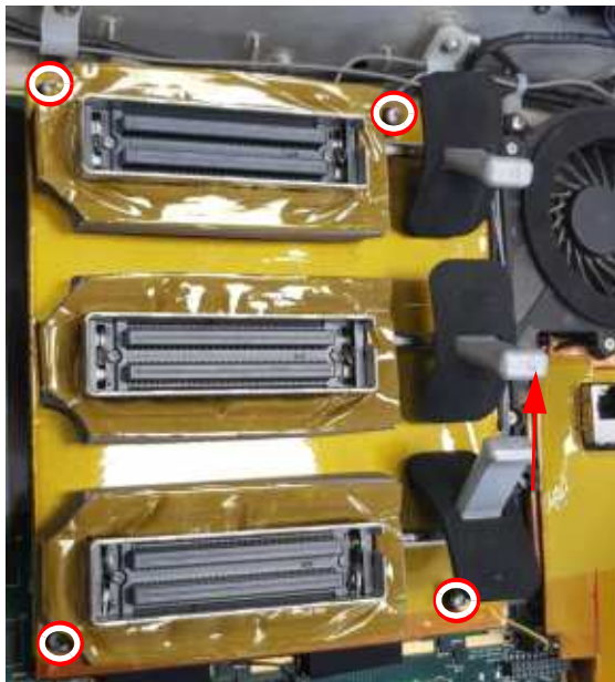
Figure 8-78 Removing Four PSB Screws
