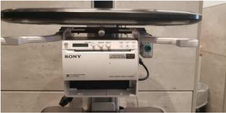
Figure 8-127 Remove Printer Assembly from the cart
