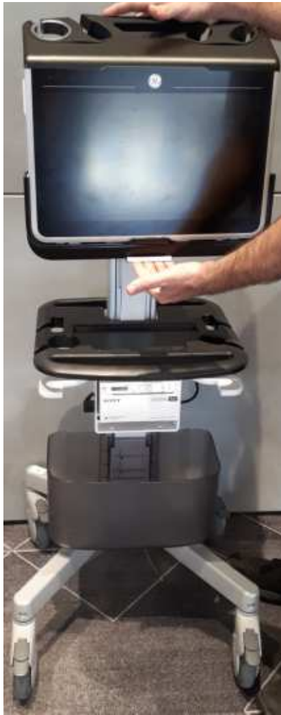
Figure 8-116 Pull Lever to Dismount System
