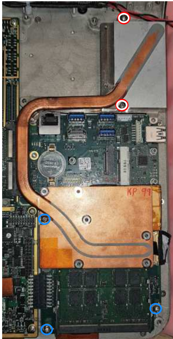
Figure 8-99 Removing 6 C-BEB Holding Screws
