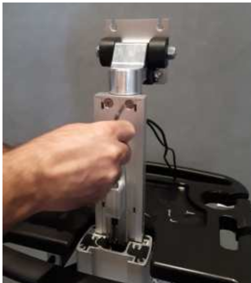
Figure 8-123 Removing Cradle Holding Screws
