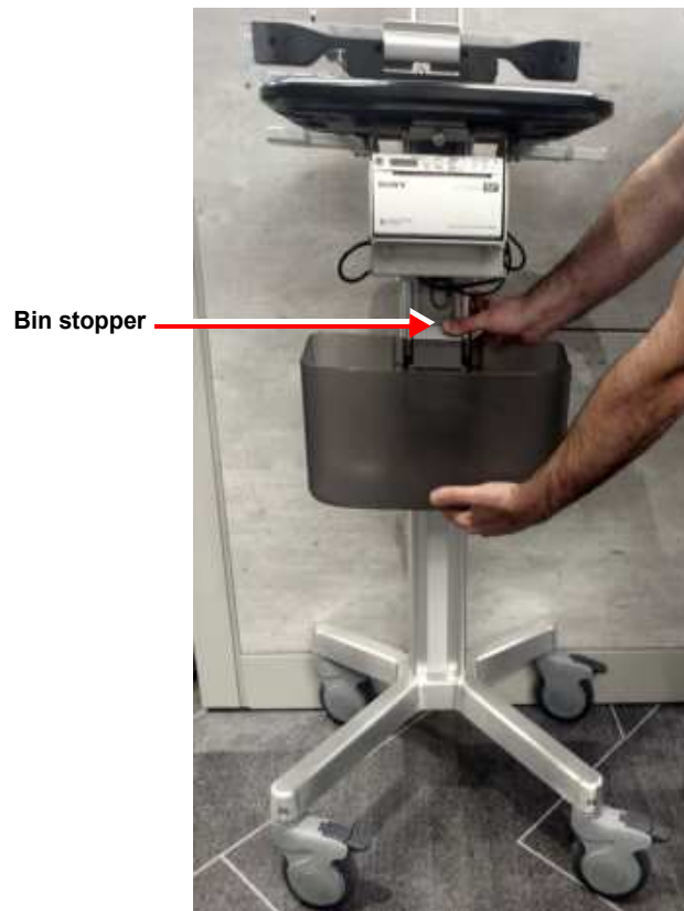
Figure 8-114 Removing Cart Bin
