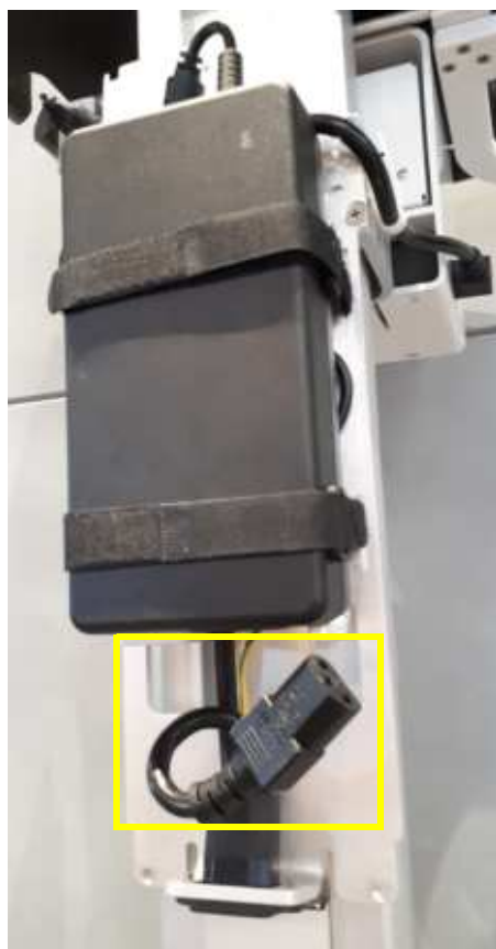
Figure 8-144 Disconnect Cable underneath Power Supply
