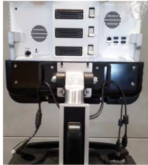
Figure 8-115 Disconnecting Cables from System
