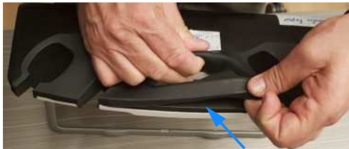
Figure 8-73 Probe Holder Rubber Removal
