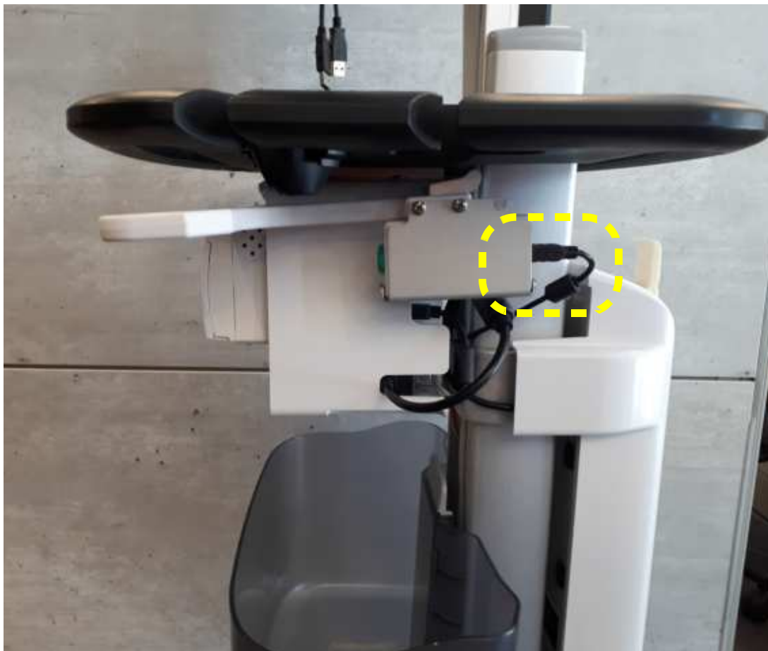
Figure 8-134 Disconnect ECG USB cable
