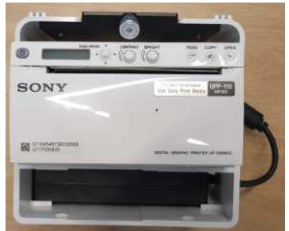
Figure 8-127 Remove Printer Assembly from the cart
