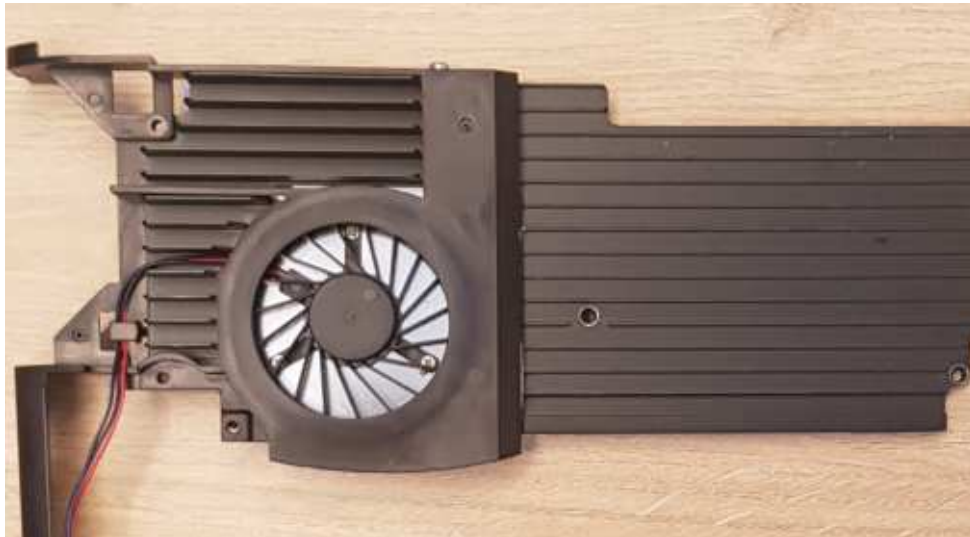
Figure 8-105 Remove the C-FEB
