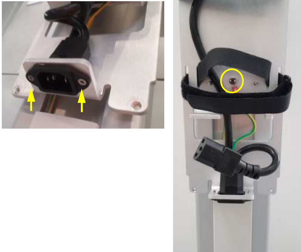
Figure 8-147 Disconnect Split cable
