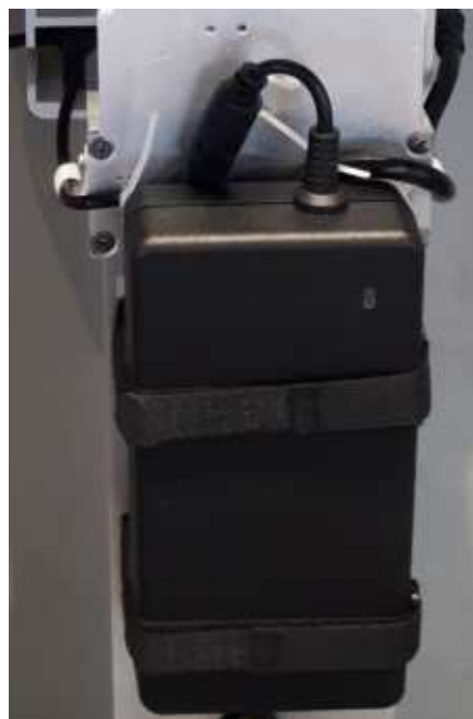
Figure 8-145 Release power cable from P clip
