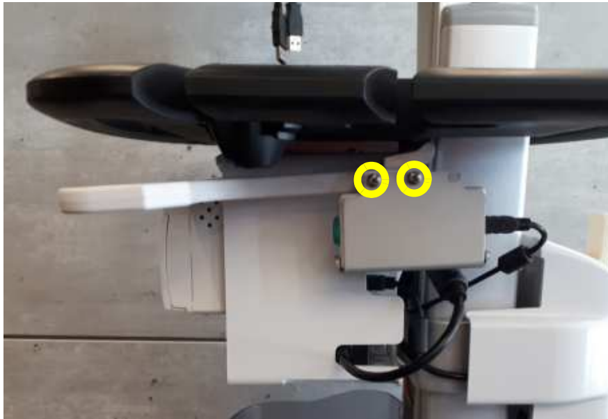
Figure 8-135 Remove ECG Bracket Screws
