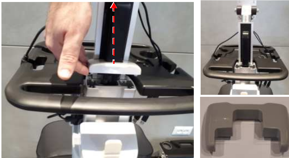
Figure 8-121 Removing Column Cover
