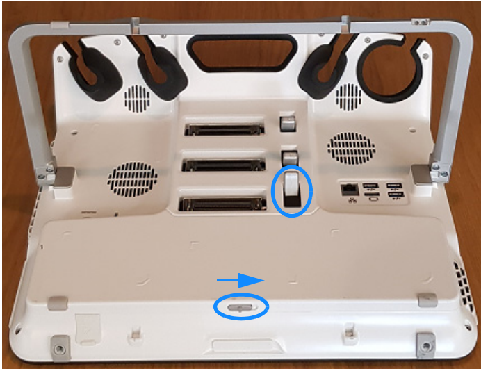
Figure 8-72 Opening Battery Compartment Cover
