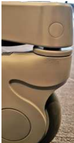
Figure 8-125 Removing Cater Cap and Holding Screw
