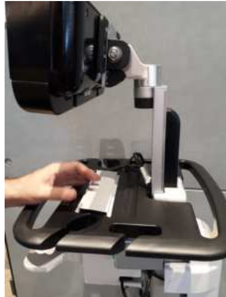
Figure 8-141 Remove Cable Plastic Cover
