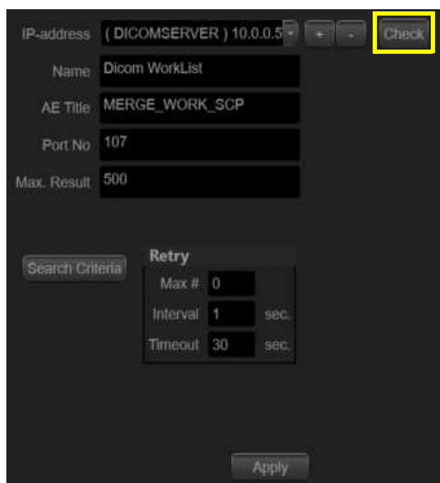
Figure 3-26 Verify Connection to a Device
