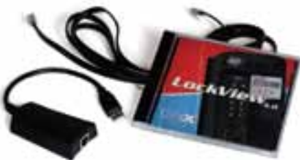
41052 – LockView Software and Dongle with RJ-11 Cable allows use to interact with electronic lock through laptop computer to perform mass programming and viewing of audit trail.
