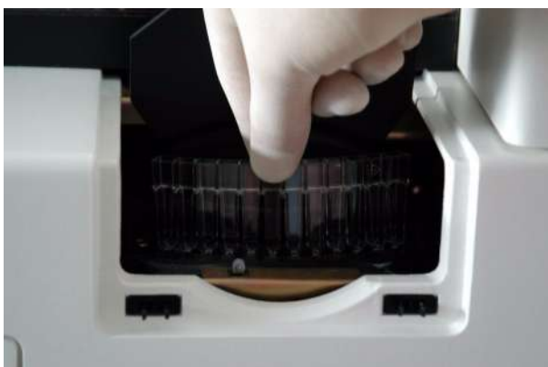
Fig. 8-12: Manual loading of cuvette segments
