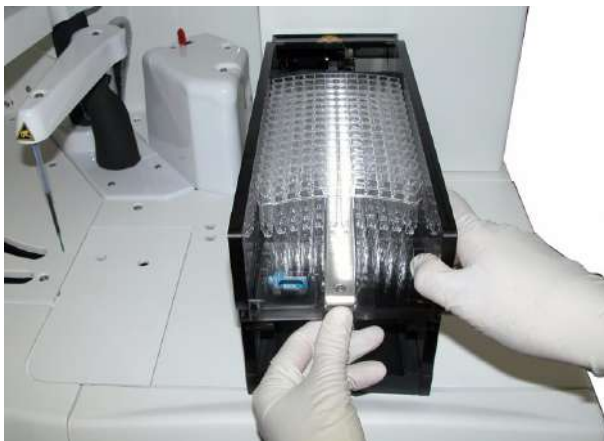
Fig. 8-11: Empty the rack of used cuvettes
