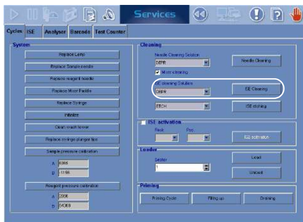
Fig. 9-4: ISE module cleaning
