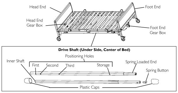
FIGURE 9 Assembling/Installing/Removing Drive Shaft
