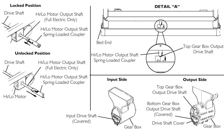
FIGURE 10 Assembling/Installing/Removing Drive Shaft
