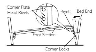
FIGURE 5 Installing/Removing Bed Ends
