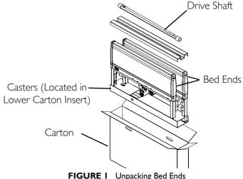
FIGURE I Unpacking Bed Ends
