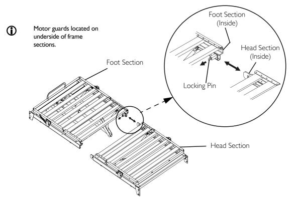
FIGURE 4 Assembling/Disassembling Head and Foot Sections
