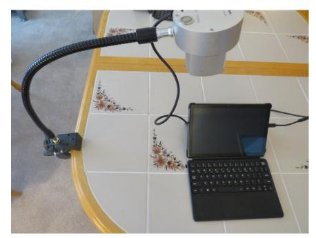
Never bend the gooseneck backwards when connected to the super clamp. If that happens, the gooseneck will break at the point where the gold adapter is attached to the super clamp.
