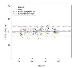
This graph shows plots of the error  $(SpO_2 - SaO_2)$  by  $SaO_2$  using the 9590 with a linear regression fit and upper 95% and lower 95% limits of agreement. Each sample data point is identified by subject from a clinical study using toes in non-motion conditions.
