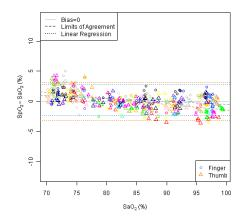
This graph shows plots of the error  $(SpO_2 - SaO_2)$  by  $SaO_2$  using the 9590 with a linear regression fit and upper 95% and lower 95% limits of agreement. Each sample data point is identified by subject from a clinical study in non-motion conditions.
