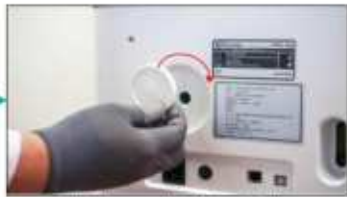
3. Slide the new HEPA filter into the hole to replace it.
