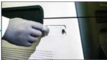
2. Remove the Knobs
