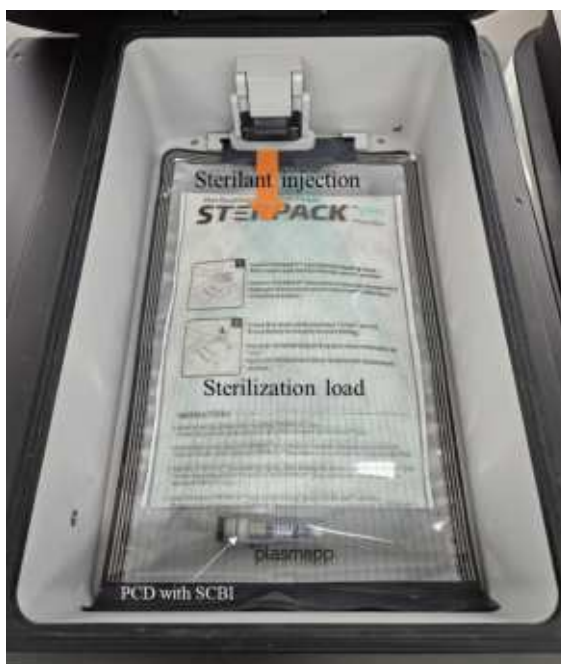
Figure 4.2 Loading STERPACK™ plus in the chamber
