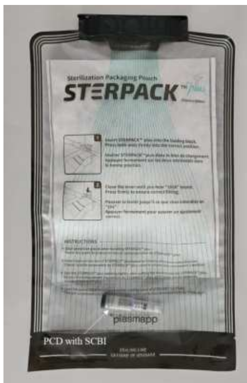
Figure 4.1 Location of PCD with SCBI in the STERPACK™ plus pouch
