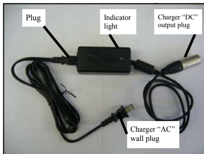
Figure 12B - Charger for P-440 lift
