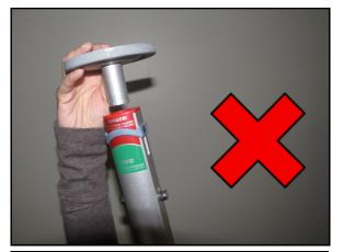
NOTE: Never install Bottom Foot at the Top section of Post
