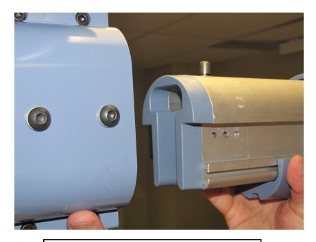
Step 18: Grab the one end of the track and slide into the swivel trolley.
