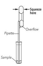
**10.** Firmly squeeze the top bulb to empty the contents of the Fixed Volume Pipette into the Cassette sample well. Extra liquid in the overflow bulb is OK.
