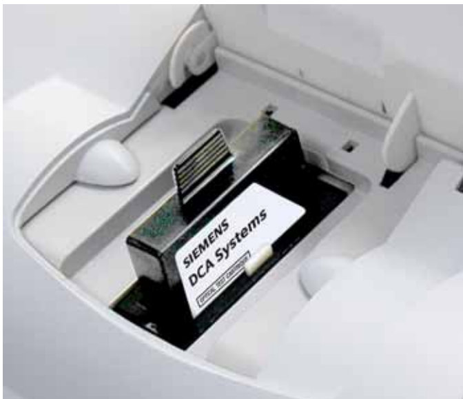
Figure 39 Inserting the Optical Test Cartridge into Compartment
