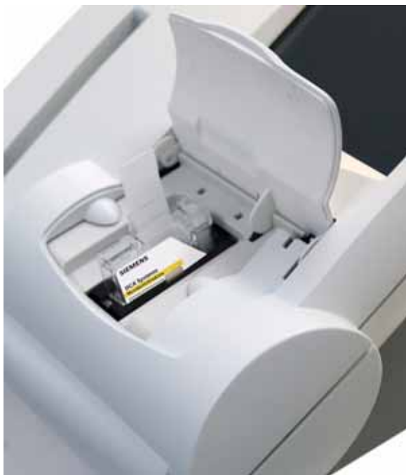
Figure 22 Inserting Reagent Cartridge into System
