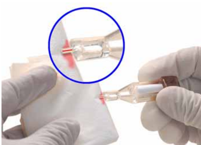
Figure 12 Wiping Outside of the Glass Capillary
