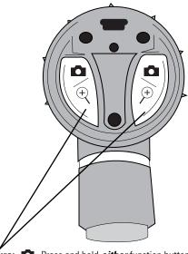
**Capture:** Press and hold *either* function button for approximately 1 second. Upon *release* of the function button the *image freezes* as a thumbnail on the screen. If the image is rotated (see below) then the captured image is rotated.
