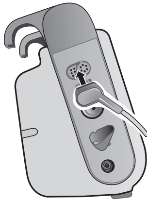
Figure 13-2 Connecting the 12-Lead ECG Cable
