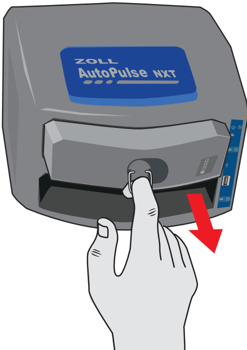
Figure 6.4. Removing the battery from the battery charger
